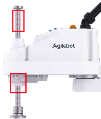
Fig. 6.4 Diagram for Greasing Area on Screw Splines
